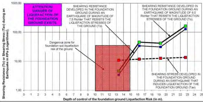
Fig. (C25). Diagram of Foundation Ground Liquefaction Risk Analysis in the location of Borehole B25.
