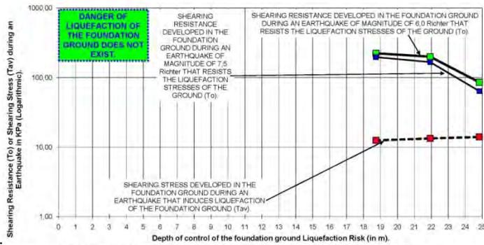
Fig. (C12). Diagram of Foundation Ground Liquefaction Risk Analysis in the location of Borehole B12.
