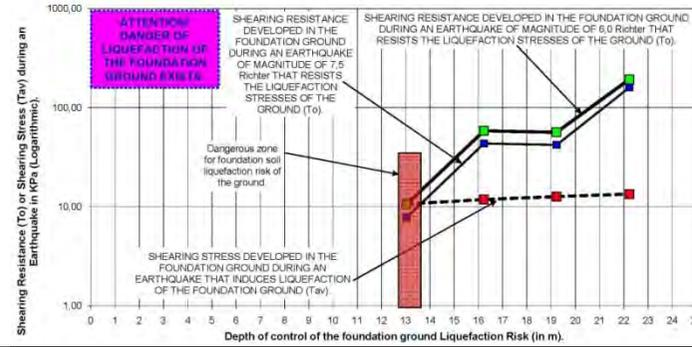
Fig. (C15). Diagram of Foundation Ground Liquefaction Risk Analysis in the location of Borehole B15.
