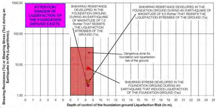
Fig. (C21). Diagram of Foundation Ground Liquefaction Risk Analysis in the location of Borehole B21.
