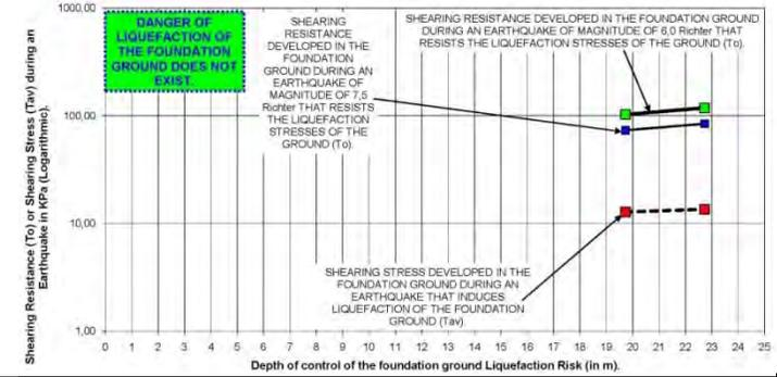
Fig. (C17). Diagram of Foundation Ground Liquefaction Risk Analysis in the location of Borehole B17.
