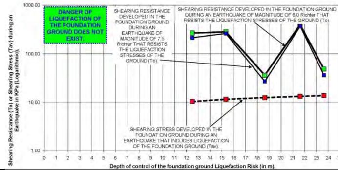
Fig. (C10). Diagram of Foundation Ground Liquefaction Risk Analysis in the location of Borehole B10.
