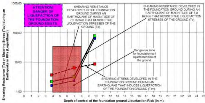
Fig. (C19). Diagram of Foundation Ground Liquefaction Risk Analysis in the location of Borehole B19.
