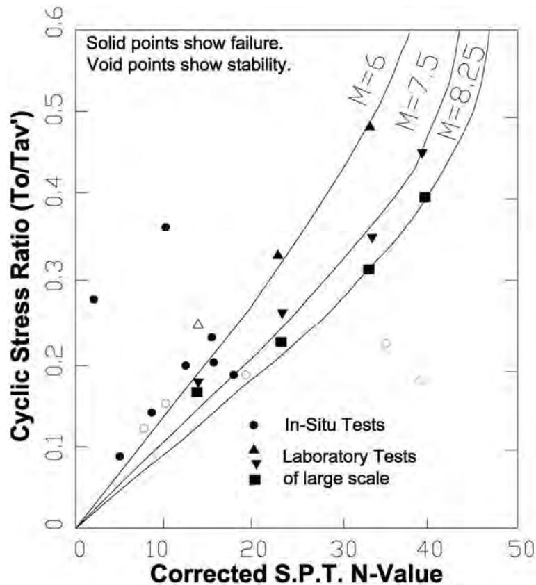
**Figure 5:** Relationship diagram between liquefaction behavior of the ground and Standard Penetration Test (S.T.P.). (after H.B. Seed, 1979).
