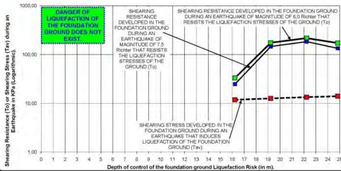
Fig. (C9). Diagram of Foundation Ground Liquefaction Risk Analysis in the location of Borehole B9.
