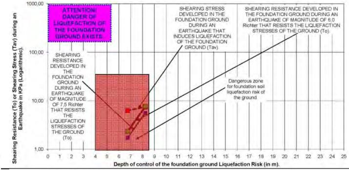
Fig. (C23). Diagram of Foundation Ground Liquefaction Risk Analysis in the location of Borehole B23.
