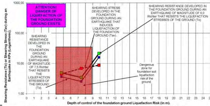
Fig. (C22). Diagram of Foundation Ground Liquefaction Risk Analysis in the location of Borehole B22.
