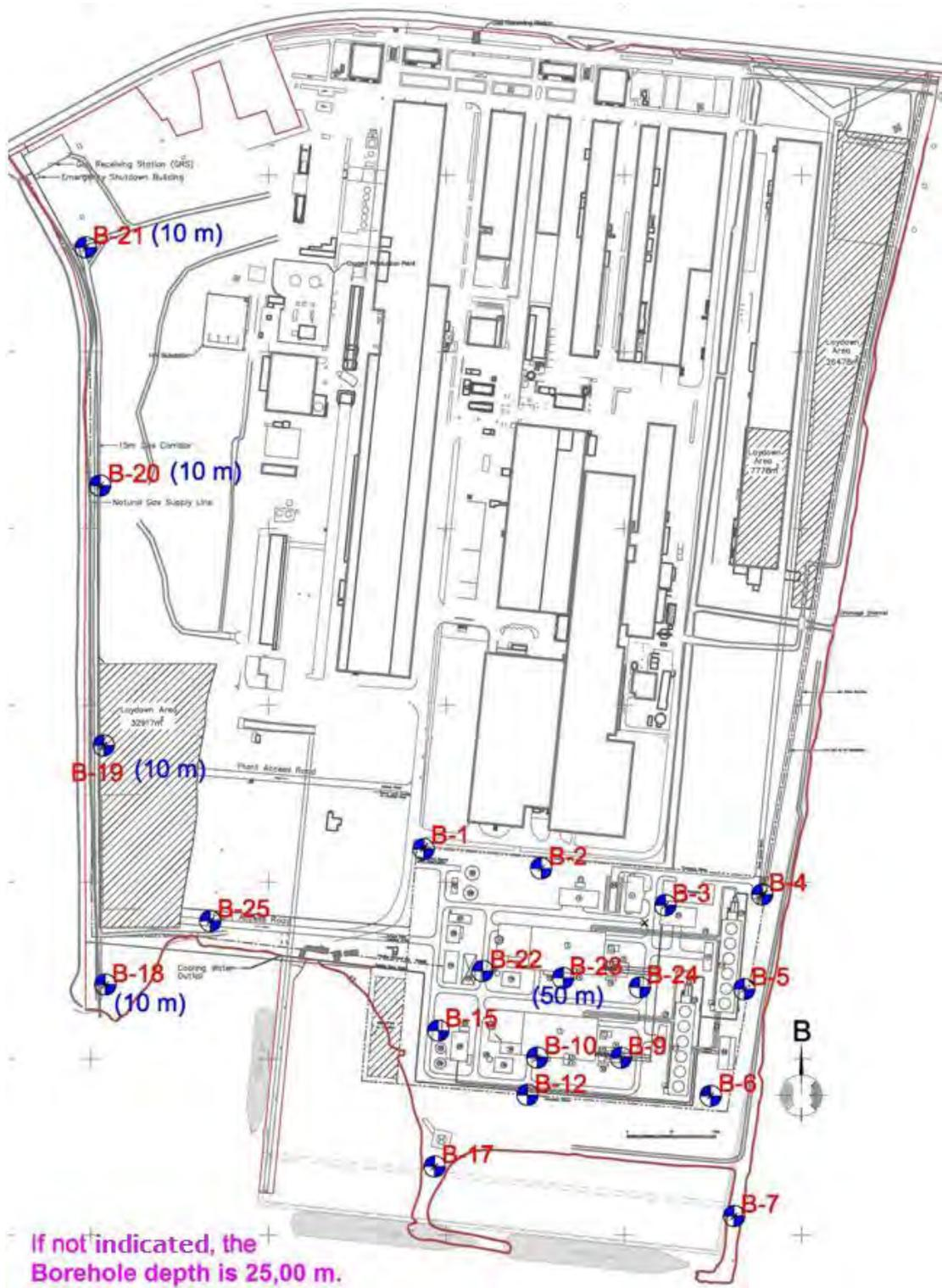
**Figure 3:** Topographic diagram showing the exact locations of the twenty investigation - sampling boreholes where S.P.T. tests were executed for the soil liquefaction potential and risk assessment, in the foundation area of the CCGT Power Plant and its pipeline alignments.
