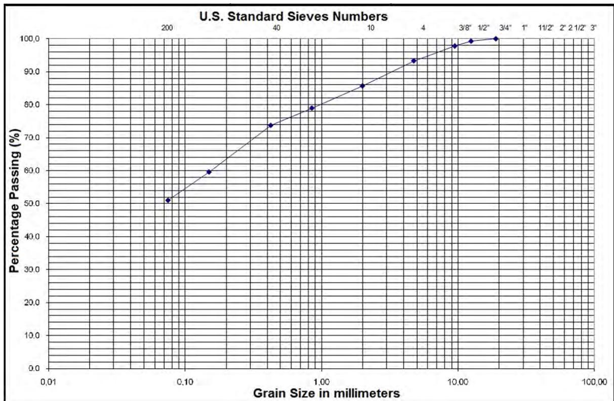
**Figure 4:** Average and typical Grain Size Distribution Curve of the layer of Silty and Sandy Quaternary Holocene Alluvial deposits.
