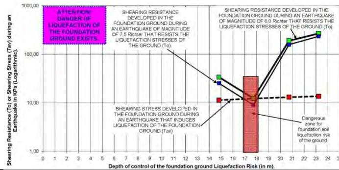
Fig. (C20). Diagram of Foundation Ground Liquefaction Risk Analysis in the location of Borehole B20.
