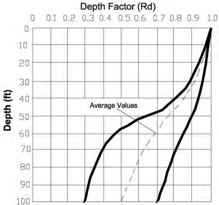
**Figure 6:** Diagram showing values of factor  $R_d$  for various types of soils in Liquefaction Risk Analysis (after S. Prakash, 1981).
