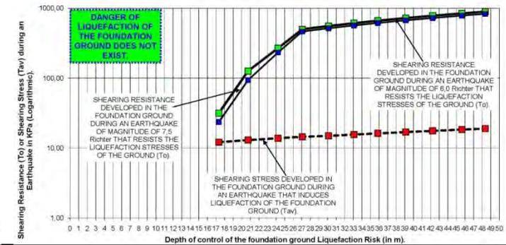
Fig. (C24). Diagram of Foundation Ground Liquefaction Risk Analysis in the location of Borehole B24.
