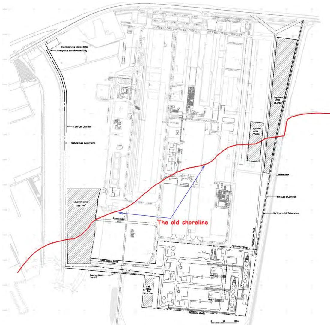
**Figure 2:** Topographic diagram showing the project foundation area in relation to the old shoreline (red line) before dumping the man made backfilling material consisting of rubble and metal objects that emanated from metallurgic furnace slag and steel block material.
