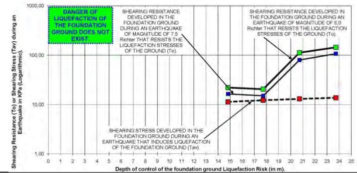
Fig. (C18). Diagram of Foundation Ground Liquefaction Risk Analysis in the location of Borehole B18.
